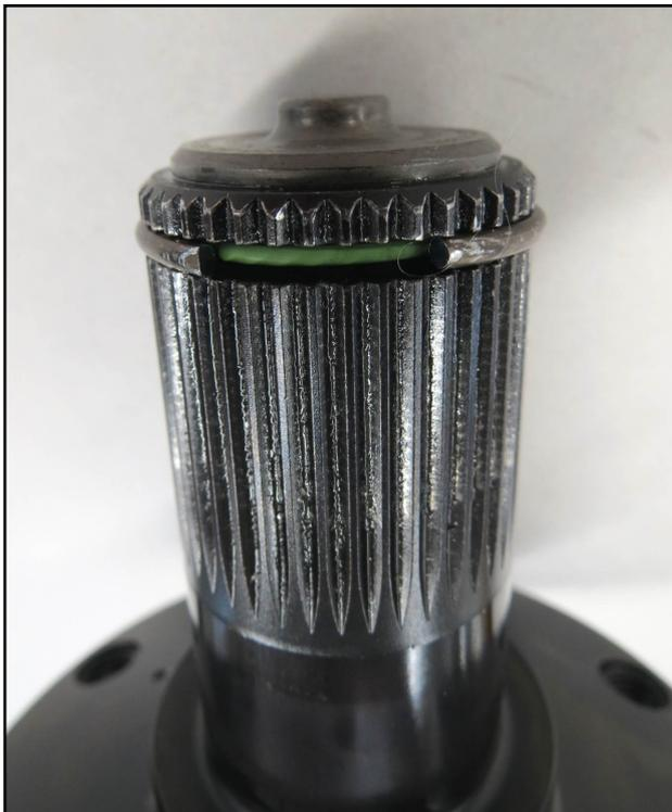
Porsche Motorsport would like to point out, that the mounting of the snap ring on the joint flange has to be done as described below. An O-ring has to be used underneath the snap ring; the procedure has to be done for both joint flanges.
